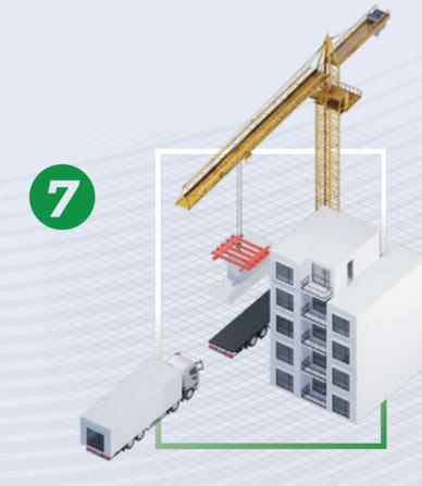
At the construction site, modules are lifted, assembled and interlocked together to form a building.
